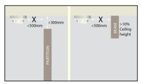
A device should not be mounted within 500mm of any obstruction. If the top of a solid partition is less than 300mm from ceiling then treat it as a wall. Similarly, ceiling obstructions such as beams should be treated as walls if deeper than 10% of the ceiling height.
