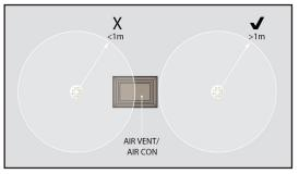
Do not site detectors less than 1m from air supply points or air circulating units.
