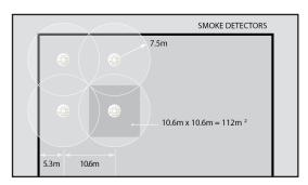
When mounted on a flat ceiling, smoke detection devices have an individual coverage of 7.5m radius. However these radii must overlap to ensure there are no 'blind spots'. Therefore individual coverage can be represented by a square measuring 10.6m x 10.6m giving an actual area coverage of 112m<sup>2</sup> per device.
