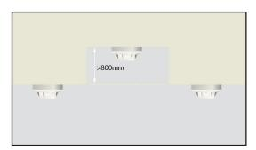
Voids less than 800mm in height need not have independent coverage, unless fire or smoke is able to spread from one area to another through the void or risk assessment shows AFD (Automatic Fire Detection) to be necessary.
