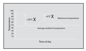
The minimum static response to heat devices should not be less than 29°C above the highest temperature the device can expect to experience.
