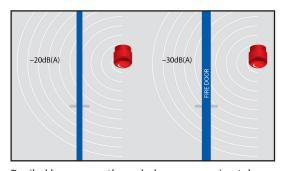
Decibel loss occurs through doors: approximately -20dB(A) through a normal door, and approximately -30dB(A) through a fire door.
