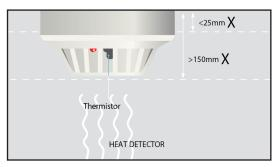
The sensing element of a heat detection device should not be less than 25mm below ceiling, and not greater than 150mm below ceiling.
