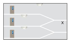
Enclosed stairways should have a detector at the top of the stairway and on each main landing.
