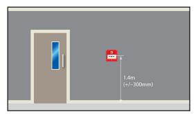
The centre of the element of a manual call point should be positioned 1.4m (+/- 300mm) from floor level. Unless a wheelchair user is likely to be the first person to raise the alarm. (Between 800-1200mm according to Doc. M. + DDA)
