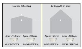
For ceilings that feature an apex: as long as the height of the apex from the rest of the ceiling is less than 150mm for heat detectors or less than 600mm for smoke detectors, then these can treated the same as flat ceilings. For higher apexes, a device should be installed at the highest point. The distance to adjacent devices can be increased by 1% per degree of angle of the roof up to a maximum of 25%.
