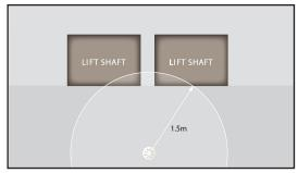
Vertical shafts like lifts and open stairways should have a device mounted within 1.5m of any opening. (This is not necessary for enclosed stairways, because as noted below, there are detectors on every landing within the stairway).
