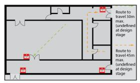
A person should not have to travel more than 45m to reach a manual call point, for a defined escape route (25m if significant proportion of occupants have limited mobility or rapid fire development is likely). For an undefined route a person should not have to travel more than 30m to reach a manual call point (16m if significant proportion of occupants have limited mobility or rapid fire development is likely).
