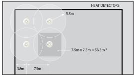
When mounted on a flat ceiling, heat detection devices have an individual coverage of 5.3m radius. However these radii must overlap to ensure there are no 'blind spots'. Therefore individual coverage can be represented by a square measuring 7.5m x 7.5m giving an actual area coverage of 56.3m<sup>2</sup> per device.
