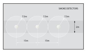
In corridors less than 2m wide the horizontal spacing of detectors may be increased, the areas of coverage need not overlap as in the case of a room. Any corridor over 2m wide is deemed a room and device spacing should follow the standard for rooms.
