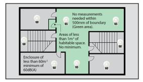
The minimum sound level should be 65dB(A) or 5dB(A) above a background noise which is louder than 60dB(A) (if lasting more than 30 seconds) and at a frequency of between 500Hz and 1000Hz. The maximum sound level should not be greater than 120dB(A) at any normally accessible point. May be reduced to 60dB(A) in stairways, enclosures up to 60m<sup>2</sup> and specific points of limited extent.
