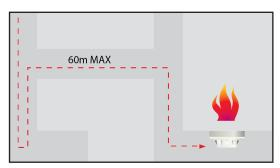
A person searching for a zone for a fire in a non-addressable fire system should not have to travel more than 60m to identify the source of a
