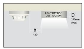
Never mount devices closer than twice the depth of light fittings or other obstructions on the ceiling.
